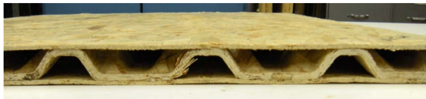
Figure 3. Sandwich panels fabricated with thin stand plies and 3D strand core.
