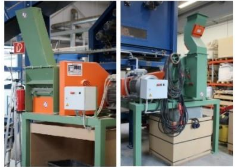
L: Chopper for chipping of solid wood R: Chipping machine for the production of middle layer material
