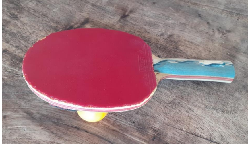
FIGURE 8.1 The composition of the plywood blade, in terms of number and thickness of layers, and wood species used, is relevant to the overall performance of a table tennis racket, which can be fast, slow, stiff, etc. (image F. Negro).
