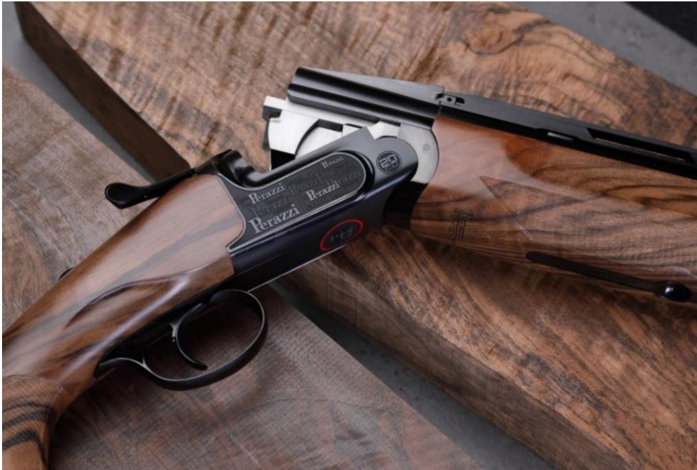
FIGURE 24.2 Rifle stocks are made starting from pieces of solid wood that often have particular figures to confer a unique aesthetic appearance to the rifle (image courtesy of Armi Perazzi).
