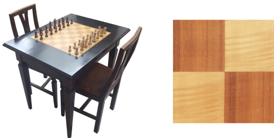
FIGURE 34.3 Left: table with an embedded chessboard; the chairs, table, chessboard, and pieces are made of wood (image courtesy of Società Scacchistica Torinese). Right: waves of fiddleback wood displayed in the light-colored squares and oriented perpendicularly to the grain of the dark squares to further enlarge the contrast between squares (image F. Negro).
