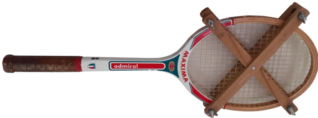
FIGURE 11.2 Wood laminated tennis rackets were produced in a wide variety of shapes and colors. Clamps were used to contrast warping during storage (image F. Negro).
