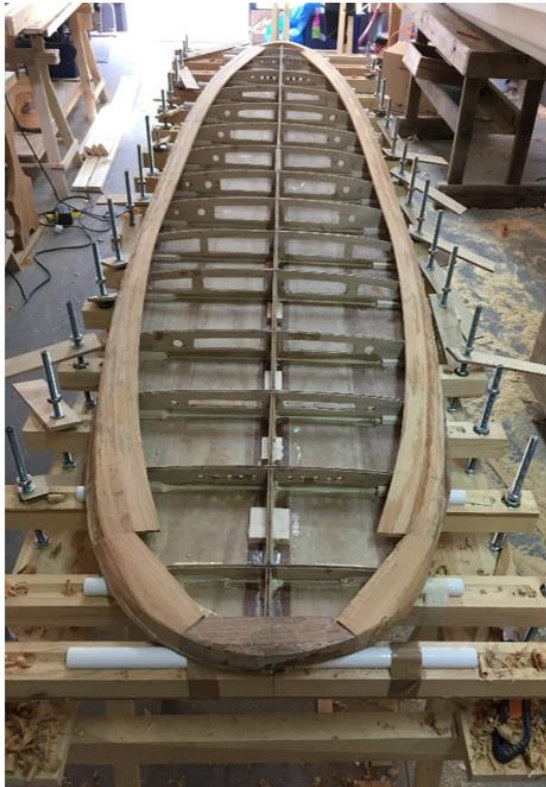
FIGURE 28.1 Wooden surfboard with a core made of thin wooden strips: on the left, during production; on the right, finished (image P. Sobotowski, surfboard produced by MIASTO SZKUTNIA, Poland).
