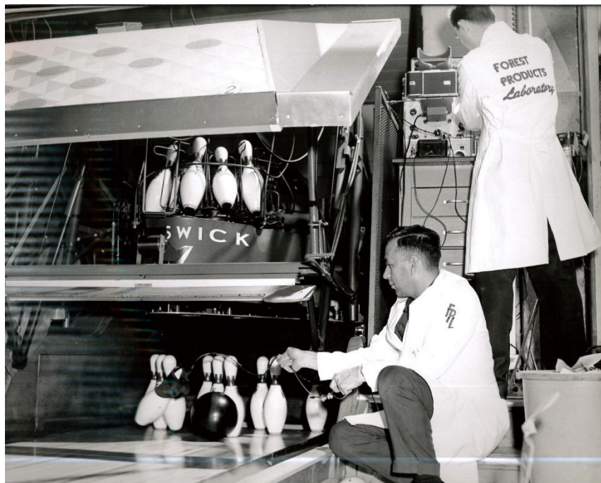
FIGURE 33.1 Strength tests conducted by Forest Products Laboratory researchers on bowling pins (image courtesy of US Forest Service - Forest Products Laboratory).
