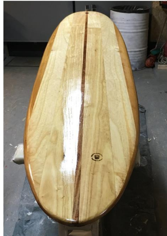
FIGURE 28.1 Wooden surfboard with a core made of thin wooden strips: on the left, during production; on the right, finished (image P. Sobotowski, surfboard produced by MIASTO SZKUTNIA, Poland).
