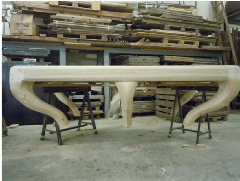
FIGURE 32.2 The EMI 54 billiard table under construction in the Rogai workshop (image G. Rogai).
