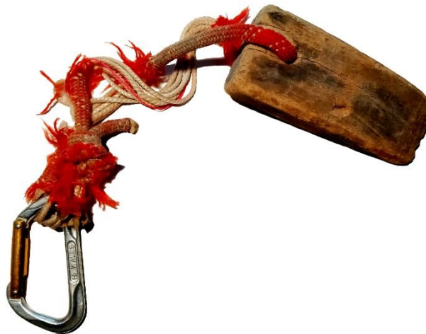
FIGURE 27.1 An old wooden wedge used to protect cracks before “friends” invention (image Flavio Ruffinatto).
