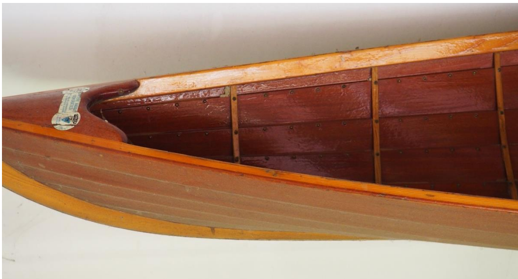
FIGURE 19.1 Example of clinker technique in an old rowing boat (image G. Goli/A. Laschi).
