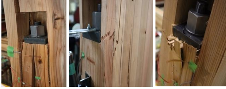
(a). Splitting failure (b). Bending failure (c). Compressive yielding Figure 11. Failure modes
